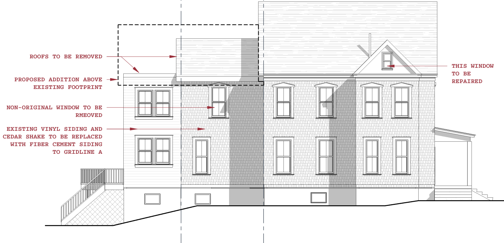
1 EXISTING LEFT ELEVATION 3/32" = 1'-0"
